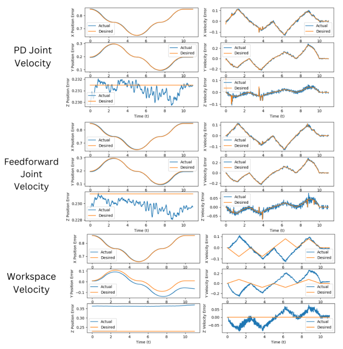
Fig. 4. Comparison between the errors in three controllers for a ten second square trajectory.
