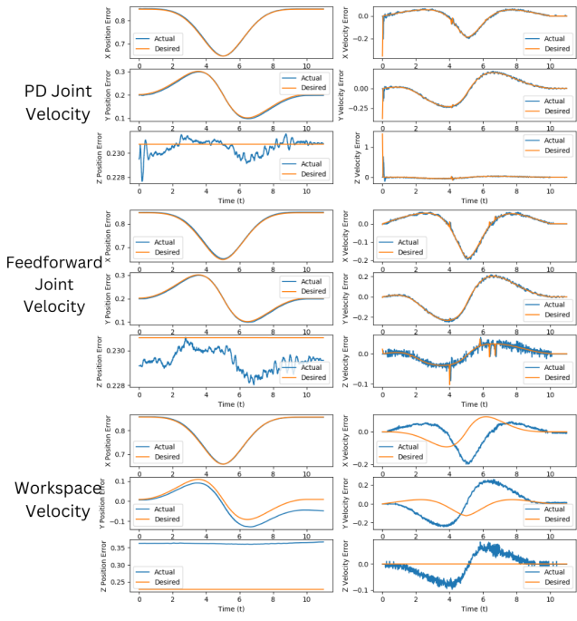
Fig. 2. Comparison between the errors in three controllers for a ten second circular trajectory.
